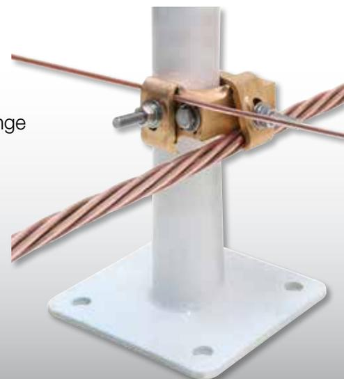
To install a SUPER-CLAMP™ connector, all you need is a half-inch socket-type tool, such as a nut driver, drill, traditional socket set, or open ended or adjustable wrenches. The “open face” design doesn’t require you to disassemble u-bolts or other hardware before installing the clamp on a pedestal.
